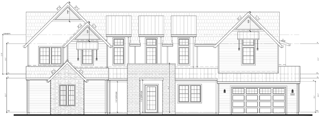
'MODERN FARMHOUSE' (COMPOSITION SHINGLE) FRONT ELEVATION 'B' 1/4" = 1'-0"
